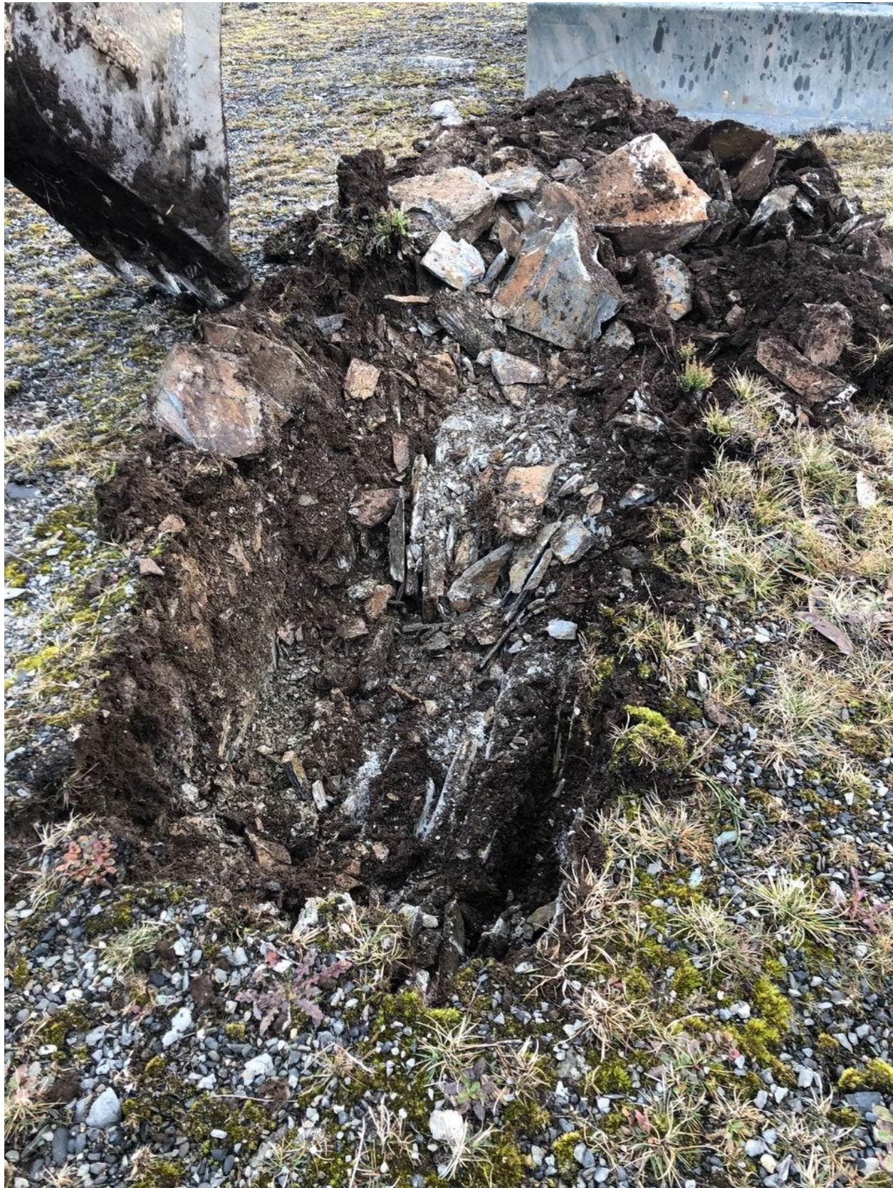
Photo 9 – 10/7/2020 – View of the subsurface profile of test pit 2T, showing shallow topsoil, directly underlain by medium strong slate bedrock.
