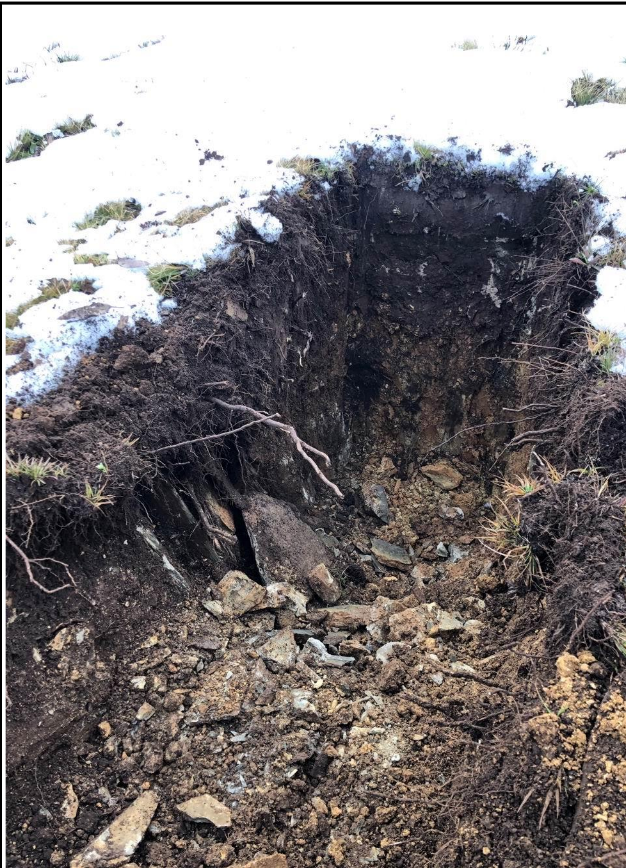
Photo 10 – 10/7/2020 – View of the subsurface profile of test pit 3T, showing topsoil, directly underlain by medium strong slate bedrock.
